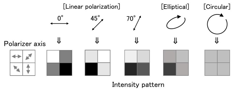
[Schematic view of polarization imaging sensor]
