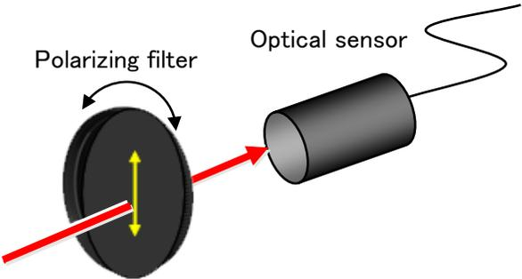
Measure of polarization is made by measuring a change of brightness when rotating a polarizing filter.
