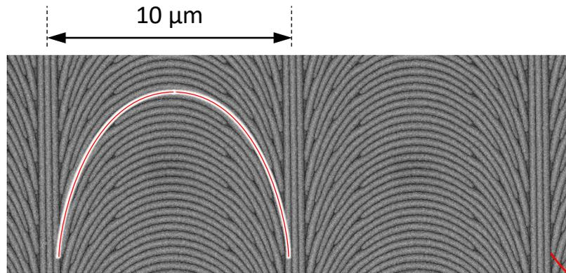
SEM image of the polarization grating surface
