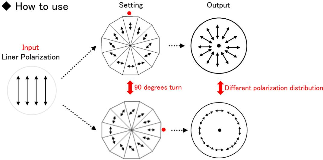
Axis symmetry polarization beam
