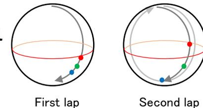
The upper limit in triple-wavelength measurement mode is bigger than measurement wavelength. It can be easily understood on the Poincaré sphere.
