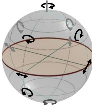
Linear polarizations are placed on the equator.
