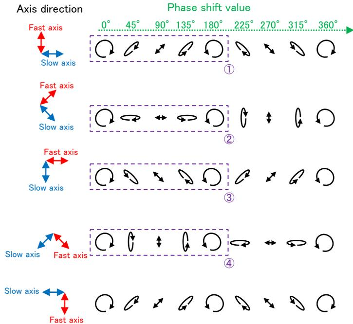
The state of polarization returns to its original state when shifted by 360-degree, for every possible direction.
