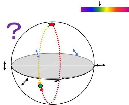
In single-wavelength measurement, we cannot distinguish a given rotation from its opposite rotation (corresponding to birefringence axis at right angle) when phase shift is greater than  $\lambda/2$ .
