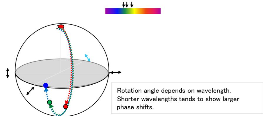
Using the dispersion of points measured at 3 different wavelengths. The real direction can be judged even when the phase shift is greater than direction where points form a line, the rotatory direction is judged  $\lambda/2$ .
