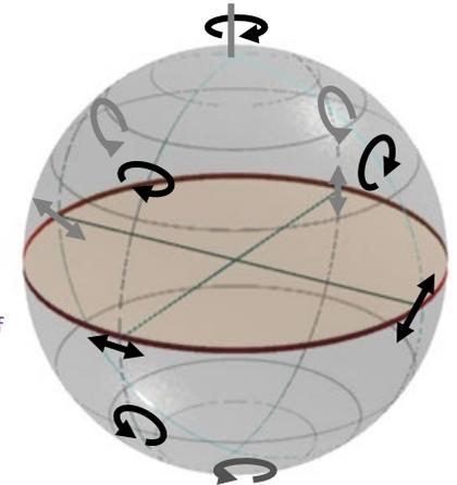
The Poincaré sphere displays each possible state of polarization as a point in a spherical coordinate system.
