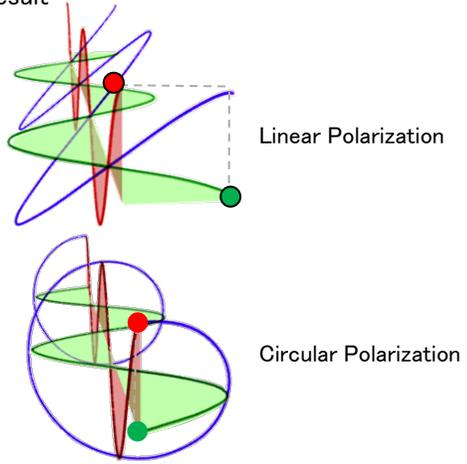
The amount of phase difference between the two components can be expressed either as an angle or as a distance, as in the relation below:
